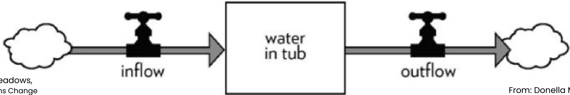
Figure 5. The structure of a bathtub system—one stock with one inflow and one outflow.
